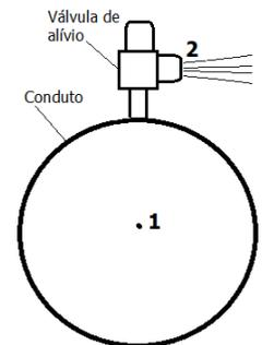
$$\frac{v_1^2}{2g} + \frac{p_1}{\gamma} + z_1 = \frac{v_2^2}{2g} + \frac{p_2}{\gamma} + z_2 + h_{1-2} \quad (1)$$
